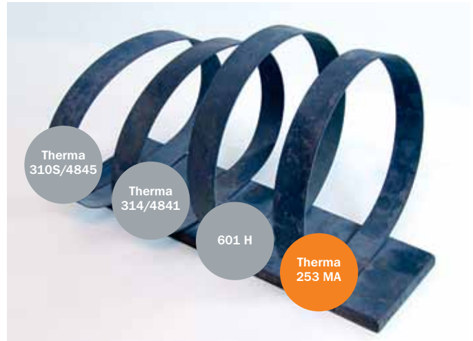
Therma 310S/4845 and Therma 314/4841 rings collapsed due to their own weight. 1000°C/1830°F, 35 hours, 1 mm/0.04 in thickness.
