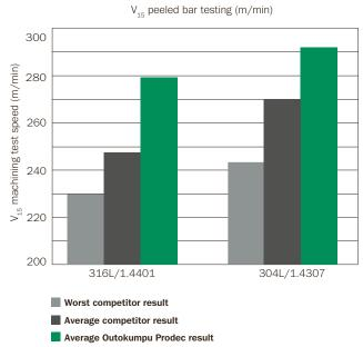
Testing done with Outokumpu Prodec and 7 European competitors' bars with improved machinability in grades 316L/4404 and 304L/4307. The tool used for testing was a CNMG 2015 cemented carbide insert.
