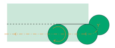
Entering the work piece can cause tool damage, especially in high alloyed duplex grades. By a soft curved entering, damage can be avoided. When passing through holes or cavities reduce cutting
