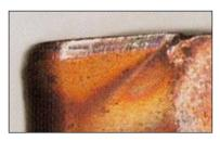
Most common in turning operations. To avoid – *reduce both cutting speed and feed.*
