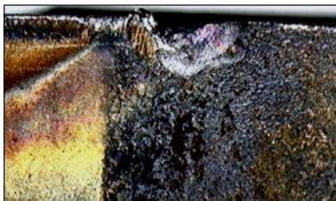
A common wear mechanism when machining in duplex stainless steel. Increased cutting speed will reduce notch but increase flank wear. If possible, use a *variable cutting depth*.
