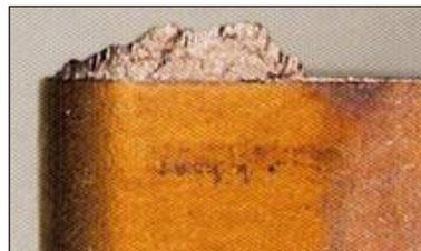
When the cutting speed is too low, the stainless steel tends to stick to the tool (in milling the chips stick to the tool). To avoid – *Increase cutting speed*.
