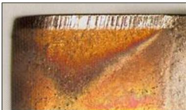
This is the ideal wear mechanism for a good and reliable machining. For longer tool life – *reduce cutting speed*.
