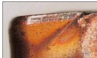
Most common in turning operations. To avoid – *reduce both cutting speed and feed*.
