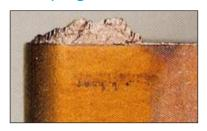
When the cutting speed is too low, the stainless steel tends to stick to the tool (in milling the chips stick to the tool). To avoid – *Increase cutting speed*.
