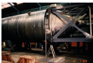
Figure 1. Kraft pulp digester (design pressure 15 bar at 200°C) in duplex type 2205 with shell thicknesses of 20-25 mm, which replaced a carbon steel vessel with shell thickness of 42 mm, i.e. weight savings of about 50%. In service 1989 [1].
