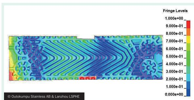
**Figure 13** Two scanned plate with different initial thickness is fitted to gather. The legend illustrates the shape deviation between components in millimeter. (NB: The picture illustrates only the middle part of the components.)
