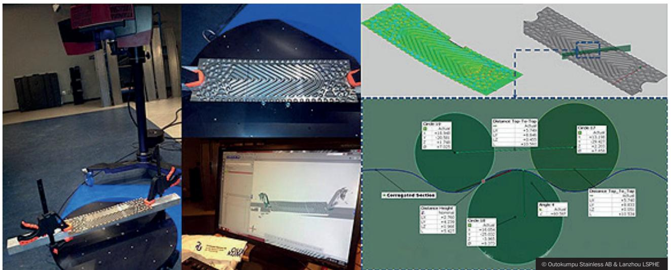
**Figure 12** Left: The set-up of the optical 3D system for the shape measurement of the PHE plate using duplex grade 2205, thickness 0.6 mm using. Right: Section based analysis and thickness distributions.
