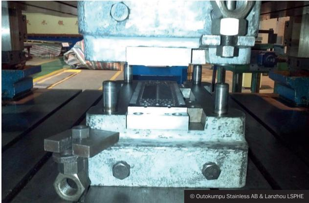
**Figure 7** Top: Press tool surface. Bottom: Tooling set-up in the press-shop
