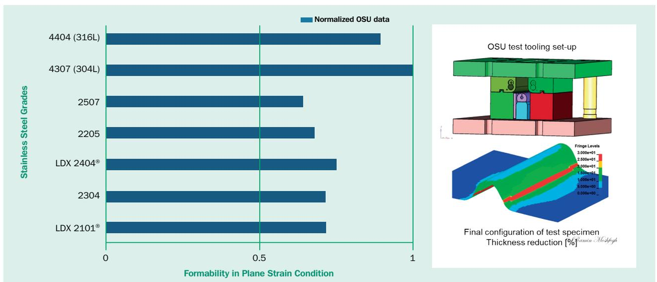
**Figure 2** OSU tooling Set-up and the normalized formability data for different stainless steel grades
