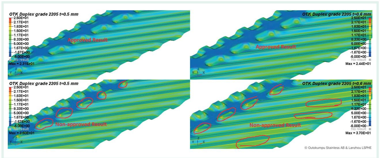
Figure 6 The numerical results from different phases of the CAE based product development with marked instabilities areas for Non-approved results.
