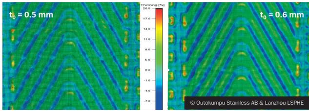
**Figure 10** The thinning distributions [%] at the final shape. Left: Duplex grade 2205,  $t_0 = 0.5$  mm. Right: Duplex grade 2205,  $t_0 = 0.6$  mm. The ranges of the legend are -10% (blue) to 20% (red).
