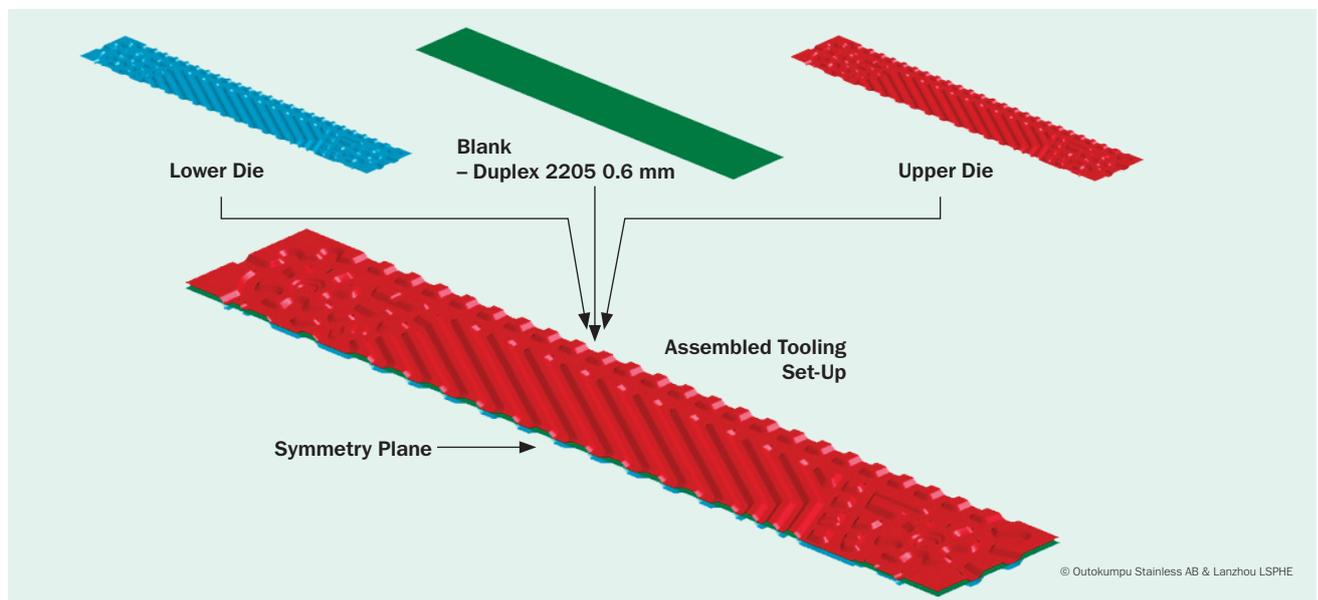
**Figure 3** The initial configuration of the press forming tools and the symmetry plane condition symmetry plane condition
