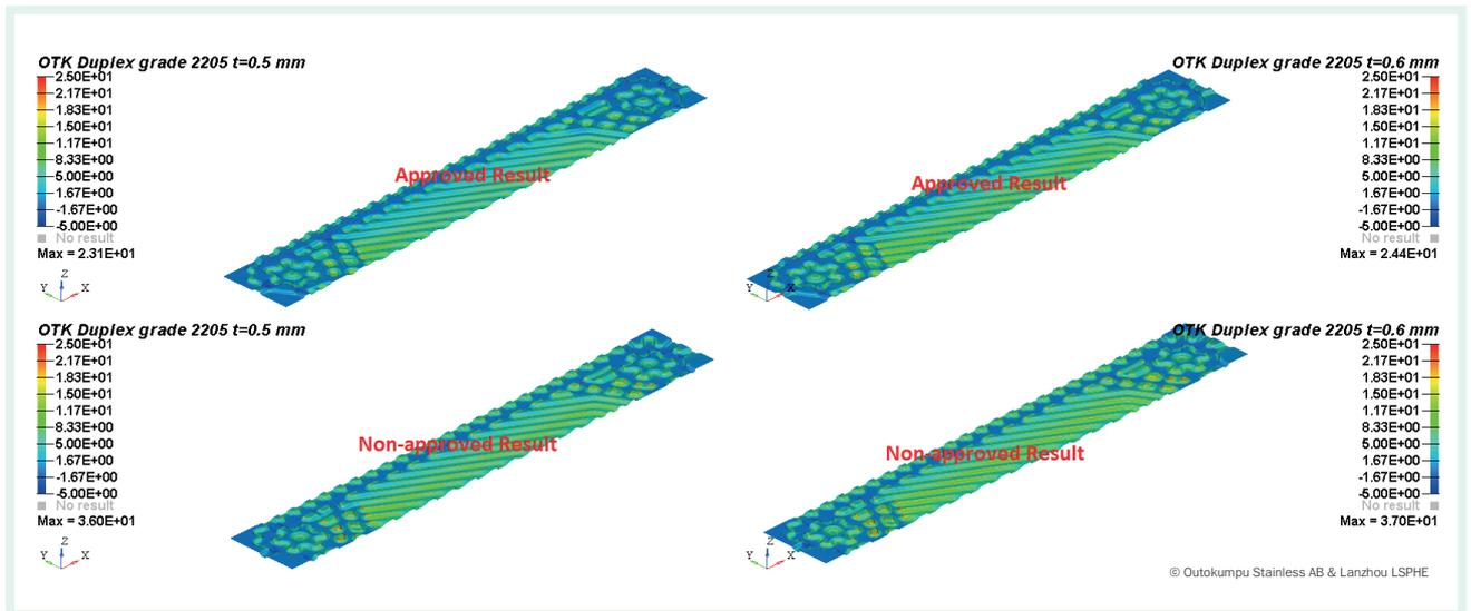
Figure 5 The numerical results from different phases of the CAE based product development. The results which are labeled with “Non-Approved results” have a thickness reduction over 30%
