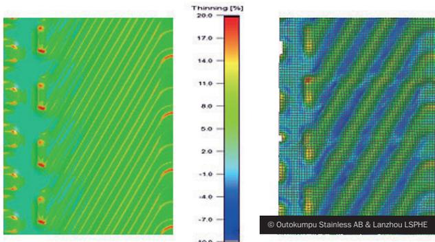
**Figure 11** Comparison between numerical results against experiment. Left: Thickness reduction according to FE analysis. Right: Thickness reduction according to strain measurements. Initial thickness  $t_0 = 0.5$  mm.
