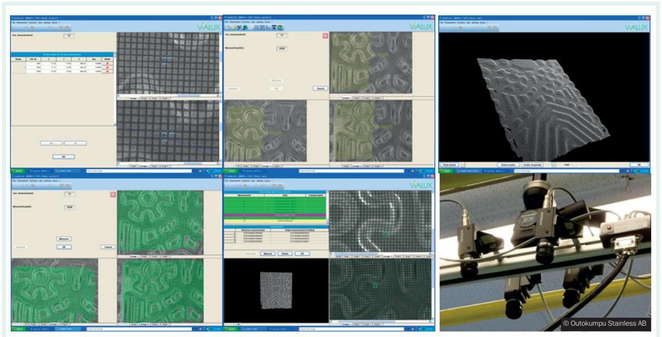
**Figure 9** Digital camera set-up and Graphic User Interface for the strain measurement
