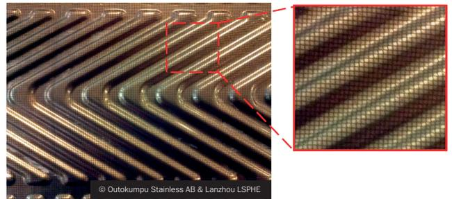
**Figure 8** The final shape of the PHE plate with gridded pattern
