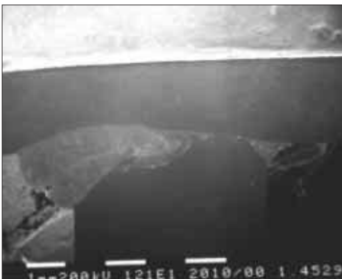
Figure 4. Section through sample of 1925 hMo plate, weld and I 625 stud.
