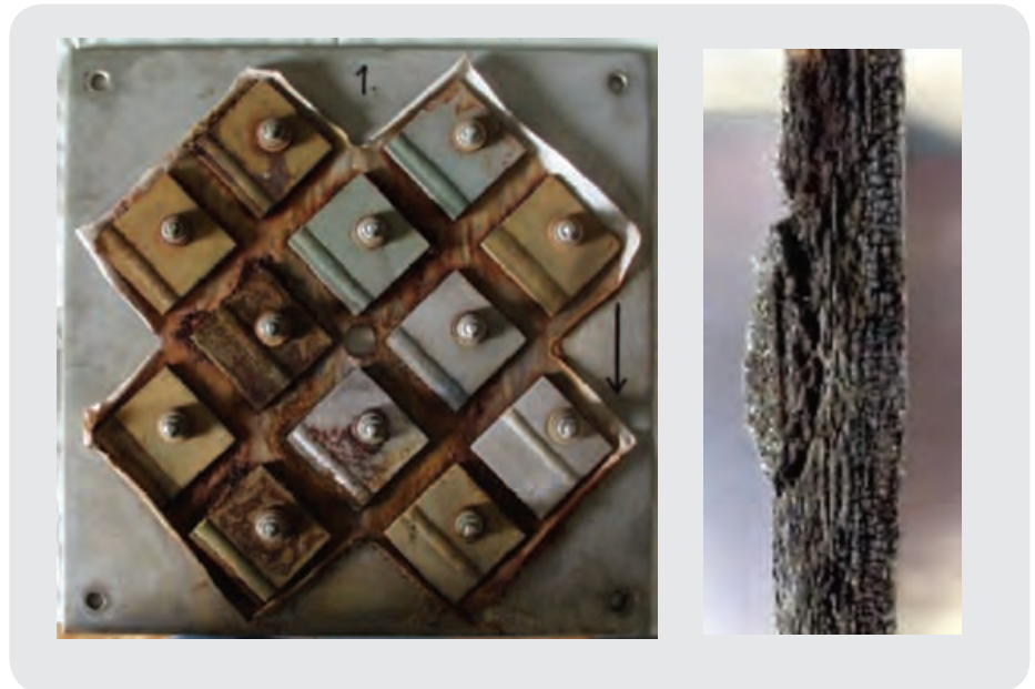
Fig. 9 Appearance of test panel after exposure for 7 months at the pre-cooler inlet and section of 2507 specimen showing corrosion in the fusion line.
