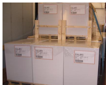
Upper layer blocked with boards and battens
