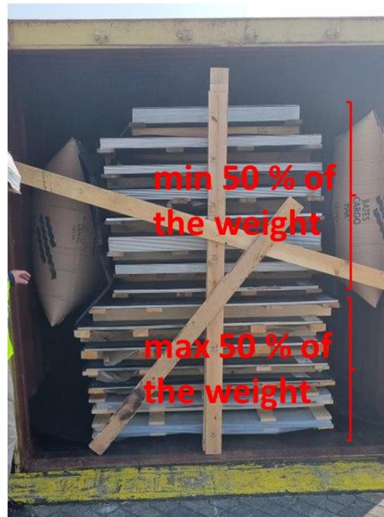
Blocking of upper layers with at least 50 % of the weight in the cargo section.
