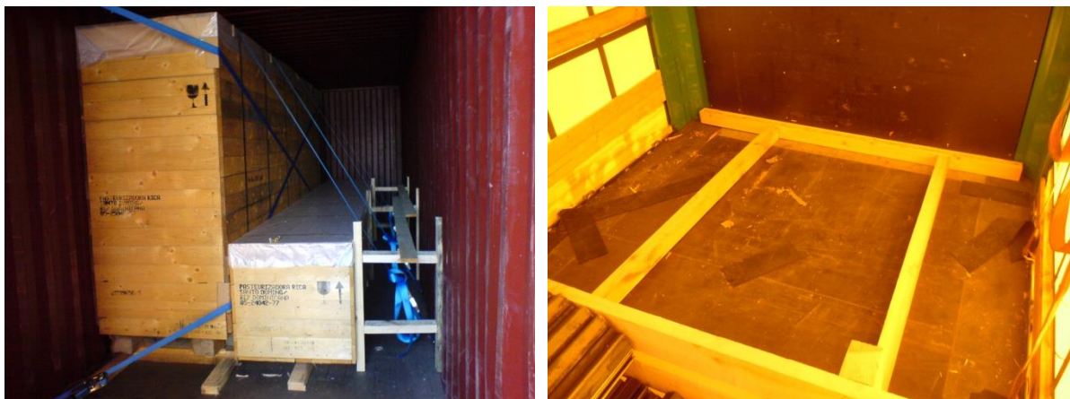
Wooden constructions for the blocking of cargo
