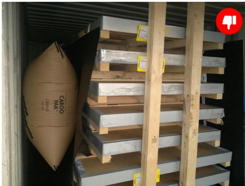
Don't put dunnage bags in too large void spaces, since this results in a very small contact area against the wall and cargo units.
