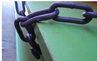
Broken links due to bending over at sharp corners
