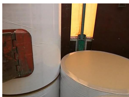
Threshold created by using cargo units with different heights
