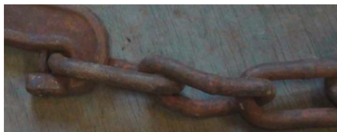
Example of damaged chain link that means that the chain cannot be used
