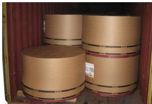
Threshold created by using empty pallets under cargo units with the same height
