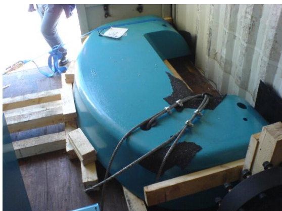
Blocking of machinery parts with timber
