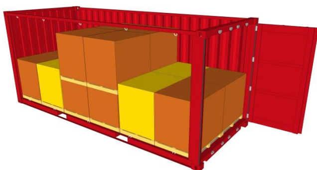
Threshold created by using cargo units with different heights
