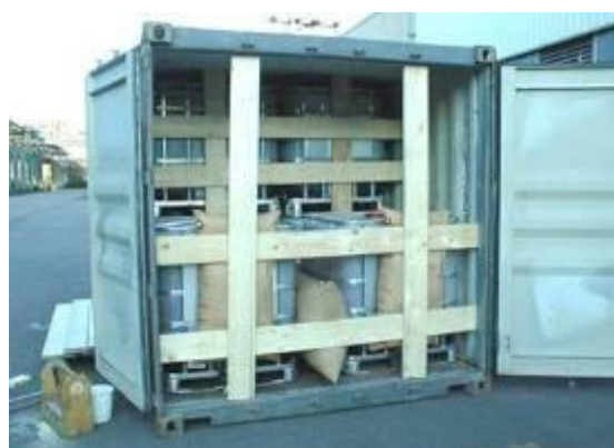
Blocking with dunnage bags and timber
