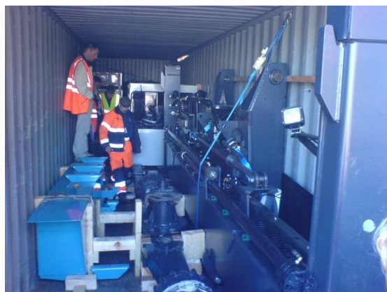
Blocking of machinery parts with timber
