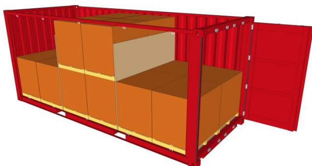
Upper layer blocked with boards and battens
