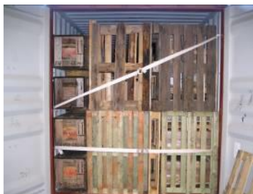
Blocking with empty pallets
