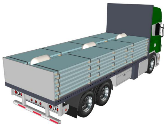
Cargo loaded against the headboard, tightly stowed throughout the length of the vehicle and blocked sideways by dunnage bags and the side walls of the vehicle (note that the side wall is transparent in the illustration)
