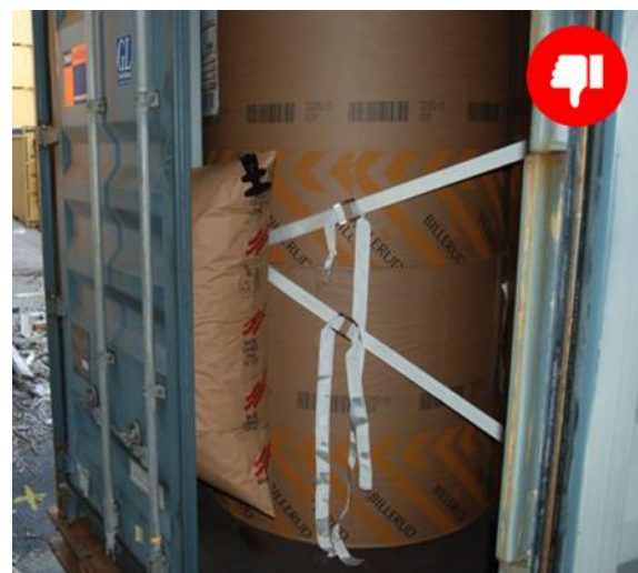
Don't put dunnage bags directly against the doors
