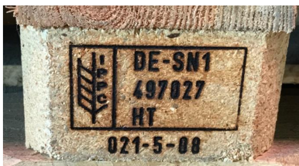
Example of marking of wood that has been heat treated
