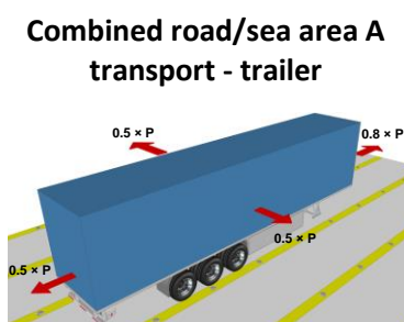
Dimensioning accelerations for the transport of semi-trailers and swap bodies in combined road/sea area A and B transport and containers in combined road/sea area C transport (please note that for sea transport a combination of horizontal and dynamic vertical accelerations might be the dimensioning case)
