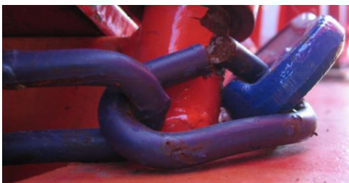
Broken links due to bending over at sharp corners
