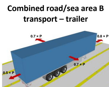
Dimensioning accelerations for the transport of semi-trailers and swap bodies in combined road/sea area A and B transport and containers in combined road/sea area C transport (please note that for sea transport a combination of horizontal and dynamic vertical accelerations might be the dimensioning case)
