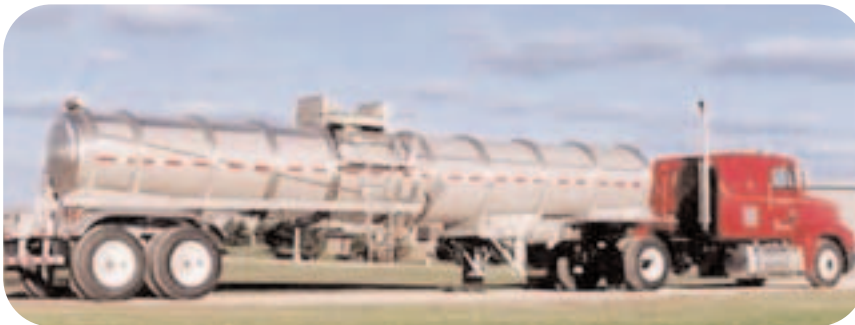
A new generation of cargo tanks from Brenner Tank will use Outokumpu's LDX 2101 rather than 316L stainless.
