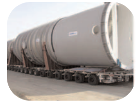
This is the first completed evaporator for the Oman facility using SAF 2507®.
