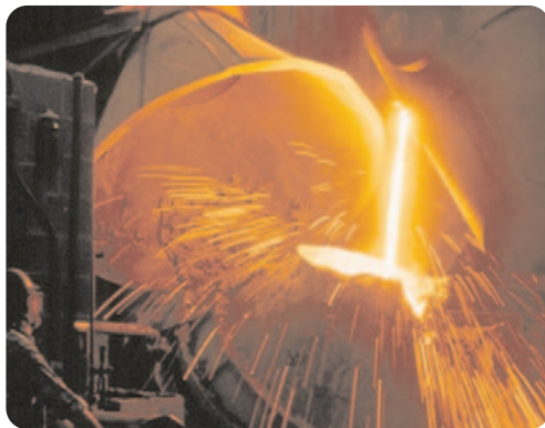
Raw materials like nickel and molybdenum are used in stainless steel melt.
