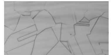
Austenite ( \gamma -iron). Face centered cubic with 12 atom neighbours. 74% close packing.
